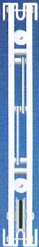
Side view of collapsible gate with a 'W' track for face and reveal fixing
